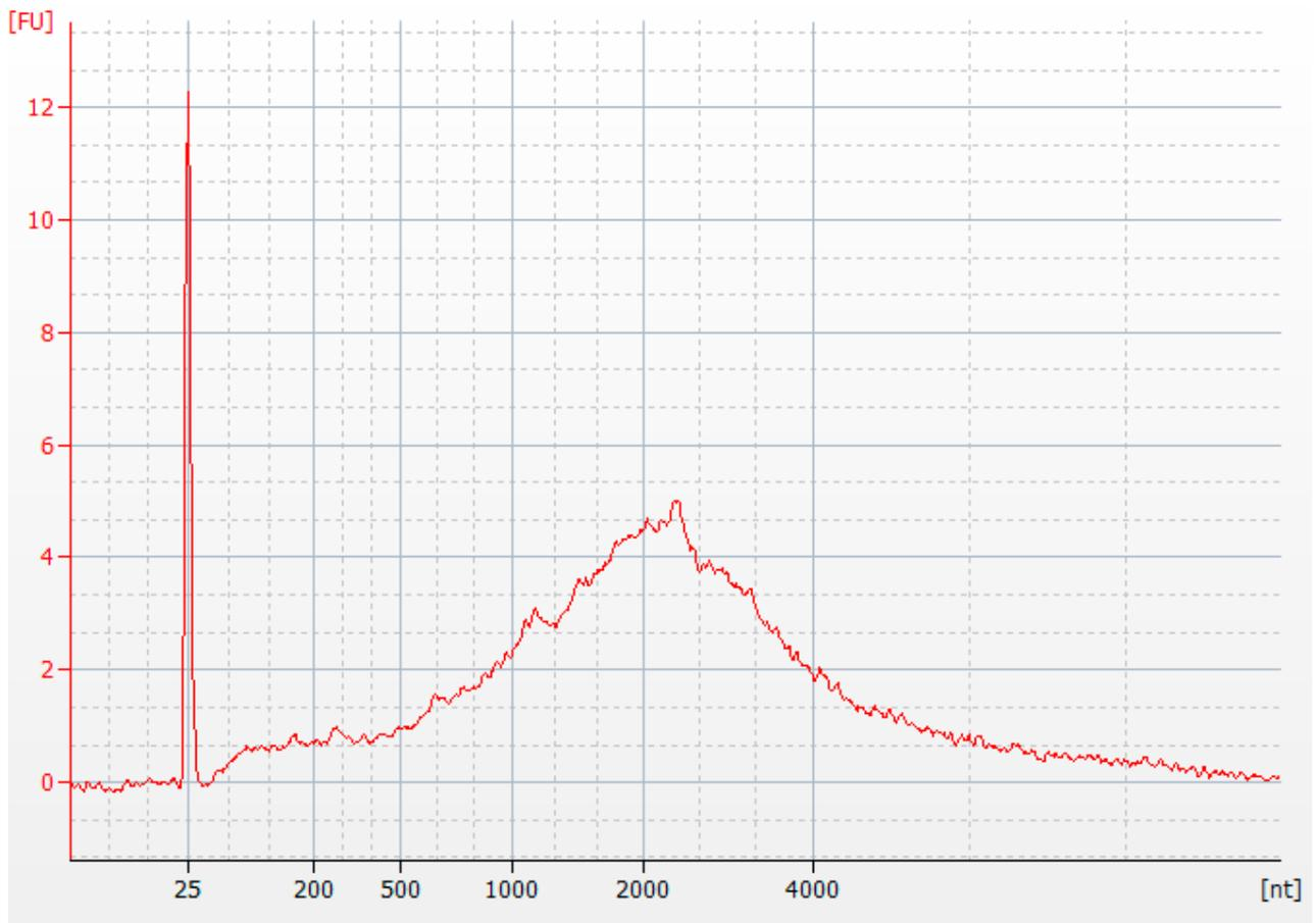
Figure 2: RNA electropherogram of poly(A) selected mRNAs after the mRNA capture from 1  $\mu$ g total Human Brain RNA (HBR) using the D-Plex mRNA Capture module (Diagenode, C05030032).
