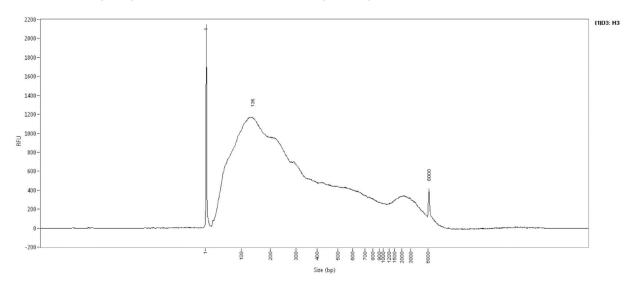
Successful chromatin shearing from HeLa cells using the Bioruptor Pico and the iDeal ChIP-seq Kit for Histones. Chromatin from HeLa was sheared using the Bioruptor Pico for 10 cycles (30" On/30"Off). Chromatin was decrosslinked and purified accordingly to the protocol for chromatin shearing analysis and fragment size was assessed using the Fragment Analyzer (Advanced Analytical).
