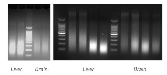
Successful chromatin shearing from mouse liver and brain using the Bioruptor Plus or Pico and the iDeal ChIP-seq Kit for Histones. Left: chromatin from mouse liver and brain was sheared using the Bioruptor Plus for 3x10 cycles (30" On/30"Off). Right: chromatin from mouse liver and brain was sheared using the Bioruptor Pico for 5 and 10 cycles (30" On/30"Off). 100 bp ladder is loaded.
