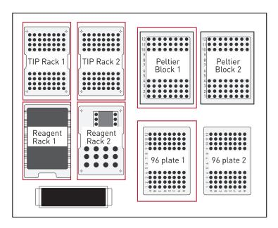
**NOTE**: The Peltier Block is now cooling down to 4°C to keep your samples cold.
