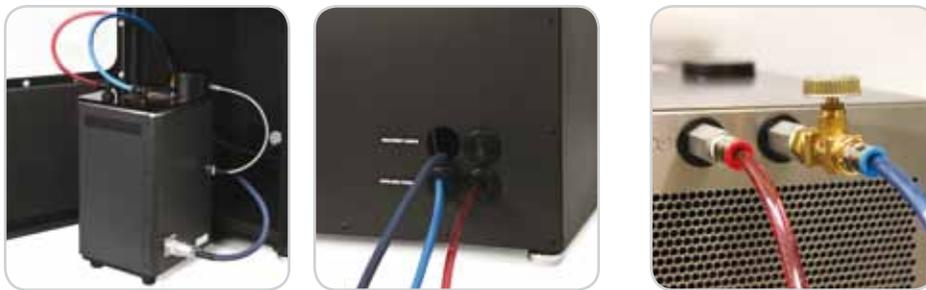
4. Position the sonication bath in front of the soundproof box upon the final site. Connect the Bioruptor® sonication bath to the Water Cooler with the red and blue tubes by inserting them in the appropriate connectors.
