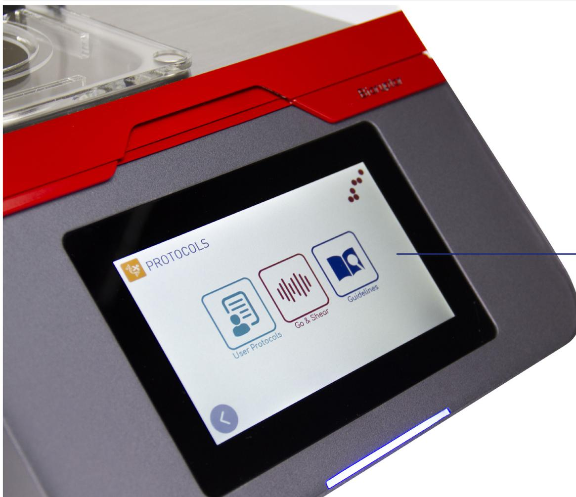
**Touch screen:** Allows the user to easily program the sonication of samples.
