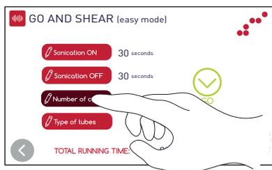
1. Enter the sonication time **ON**, the sonication time **OFF** and the number of cycles. These are the parameters controlling the shearing process:
