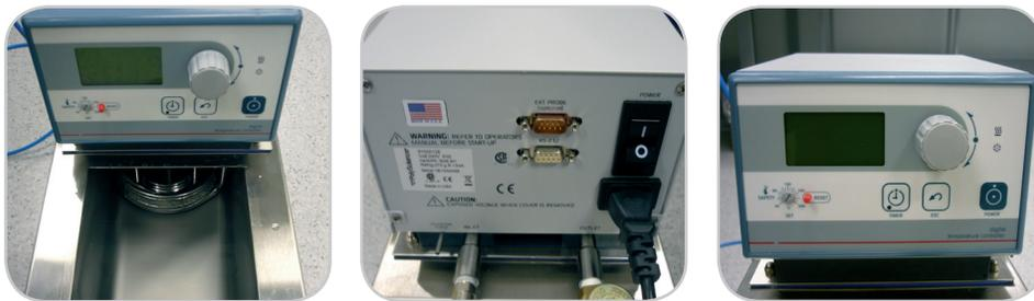
5. Fill the tank of the circulator with 4.5 litres of water. Distilled water should be used in order to minimize the proliferation of bacteria.
